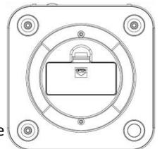
If there is no battery and the power is interrupted, the clock date/time will need to be reset.
